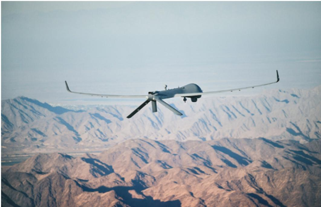
*Figure 14: Predator XP remotely piloted aircraft*
