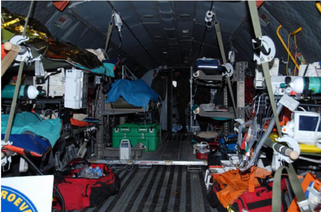
*Figure 18: Aircraft equipped for aeromedical evacuation.*
